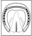
The distance from the frog apex to the inside border of the shoe should be between 1/8" - 7/8" depending on the size of the shoe (00 to 5). All shoes should extend to the end of the frog, which usually means that some shoes will extend beyond the heel buttress.
